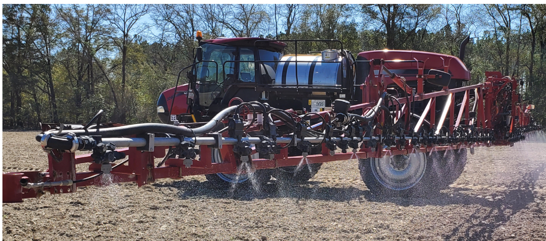
Figure 4. A PWM system using blended pulse on a sprayer boom. Observe that every other nozzle is operating at an alternate frequency.
